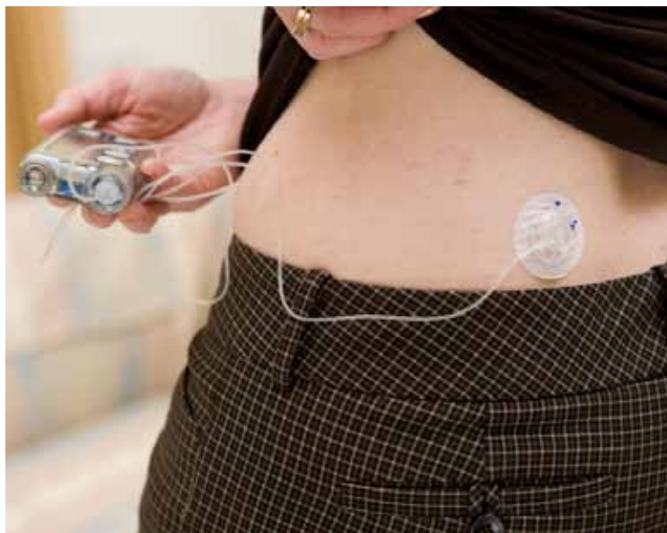
The small insulin pump automatically delivers insulin according to a programmed rate that is customized to each individual patient, and allows the patient to bolus when additional insulin is needed.
